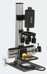
Clear stage platform with top lighting and backlighting. Can measure both reflectance and transmission.
