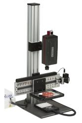
Backlighting with a clear stage platform. Often used to scan biological samples.
