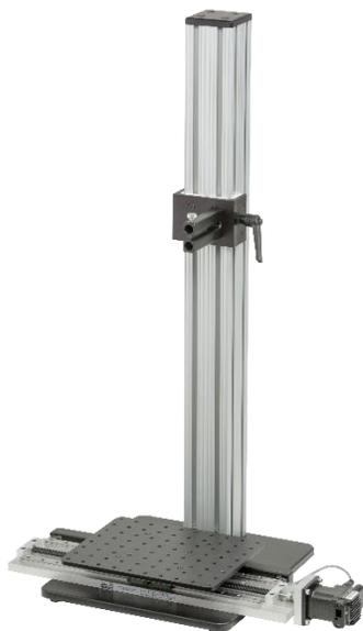
The linear stage holds the sample and translates across the field of view. Used for small samples that are easy to move.
