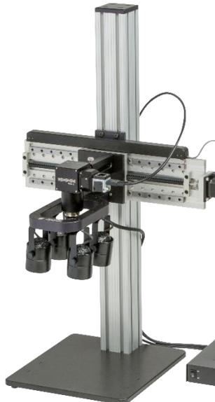
The imager and lighting assembly are mounted to the translation stage, which is mounted on the tower. Used to scan stationary objects.
