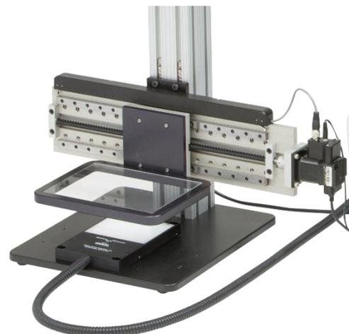
Backlighting with a clear stage platform. Often used to scan biological samples.
