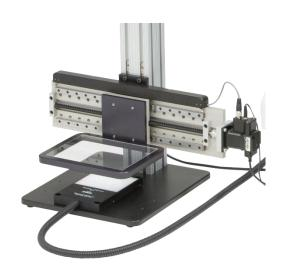
Backlighting with a clear stage platform. Often used to scan biological samples.
