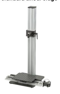
The linear stage holds the sample and translates across the field of view. Used for small samples that are easy to move.
