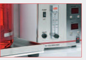
The FerMac 368 Gas Analyser measures oxygen and carbon dioxide in exit gas, two important extra parameters which give the best indication of growth within a fermenter vessel.
