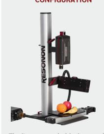
The linear stage holds the sample and translates across the field of view. Used for small samples that are easy to move.
