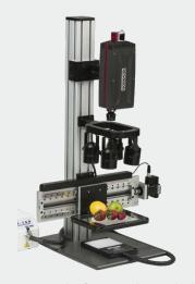
Clear stage platform with top lighting and backlighting. Can measure both reflectance and transmission.
